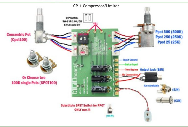
The CP-1 Compressor Limiter is an extremely versatile tool. Whether set to enhance clean picking, increase crispness and jangle, or just for all out sustain, the key to using the CP-1 is mastering its controls. The control setup is similar to a footpedal- VR2 must be pre-set, J1 and J2 are user adjustable.
